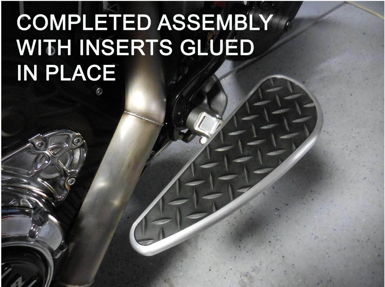
The clevises we supply are travel limited, so if the boards pivot up, they do not strike the exhaust on the right side, and the round engine cover on the left. The outside of the board is a little higher than the stock pegs, but if you ride aggressively and scrape pegs, these may scrape too, and will only pivot up a fixed amount.
